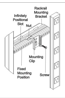
**TIP**: To remove the power strip from the mounting clips, wedge a flat tip screwdriver between side of power strip and clip, gently prying the power strip from the clip.
